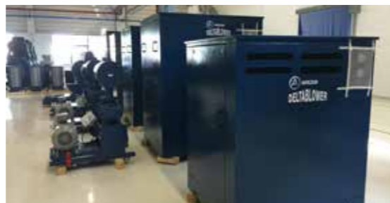
Figure 7 - Blower Package with Acoustic Hood
